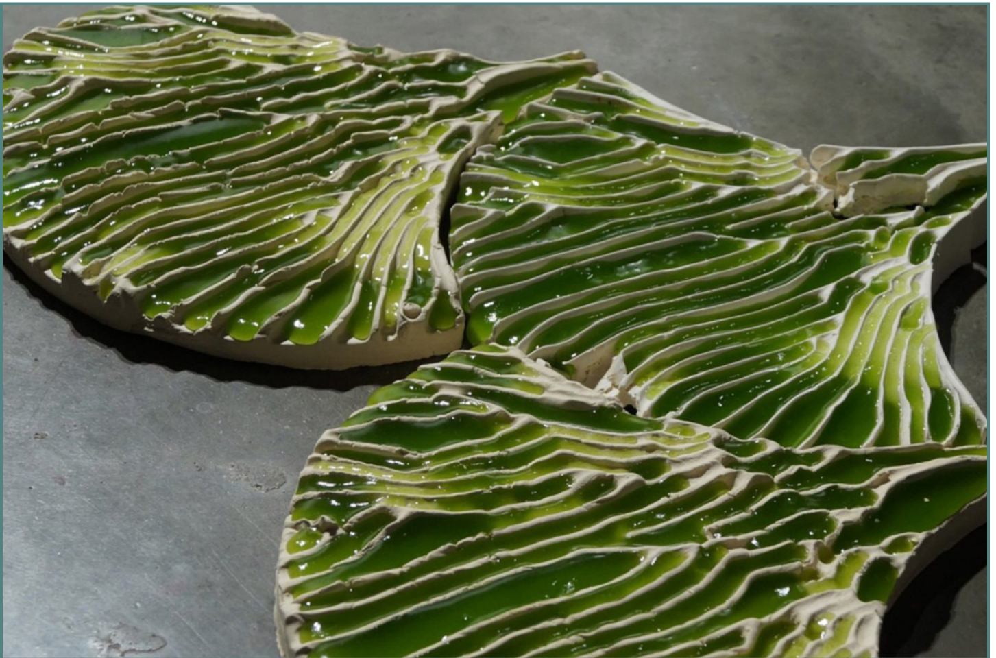
Figure 66: Toxin-absorbing algae coated tiles by Shneel Malik combines biomimicry with the tactile sense for a unique building material 475 ; Photo credit: Shneel Malik / Yanko Design
