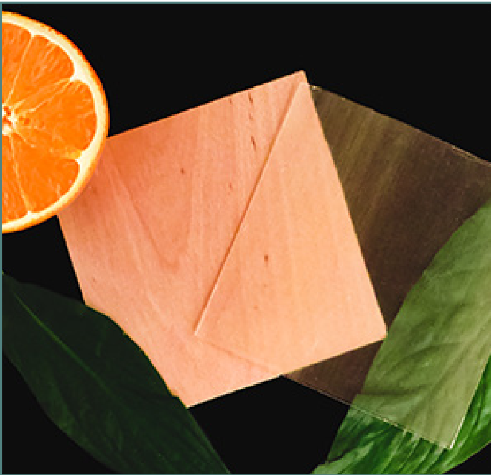
Figure 191: Transparent wood (infused with a clear bio-plastic made from citrus fruit) developed by KTH Royal Institute of Technology in Sweden; Photo credit: Céline Montanari via KTH
